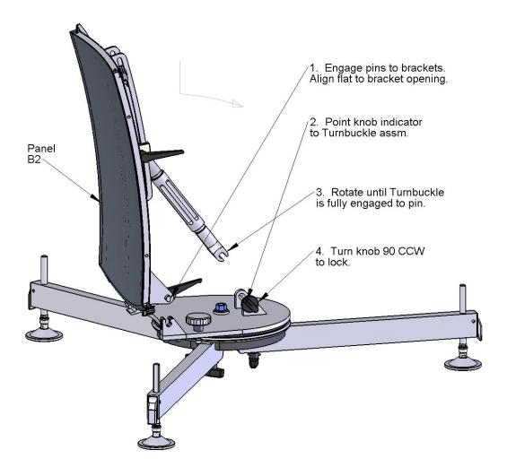
2. Adjust the Elevation to approximately 30 degrees for the installation of the remaining five panels. (Elevation scale is on back of panel B2 near Turnbuckle)
